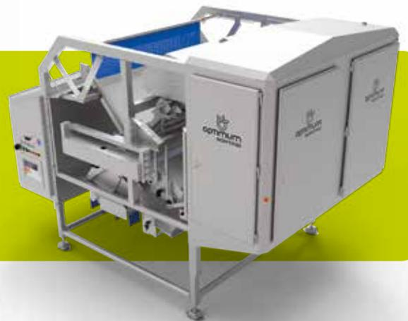
As a freefall sorter, the TRIPLUS is extremely compact. It has few moving components and therefore requires even less maintenance. Moreover, while falling, products may be viewed along two opposite sides, resulting in more accurate sorting.
